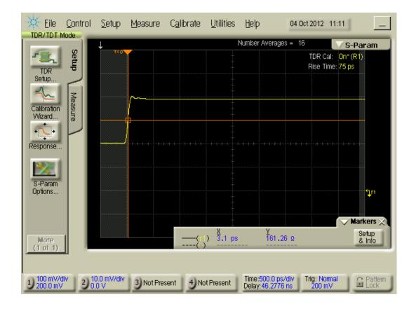
FLASH-SHORT establish the time reference plane perfectly aligned with DUT launch plane. Refer the grey area aligned with step pulse rising edge.
