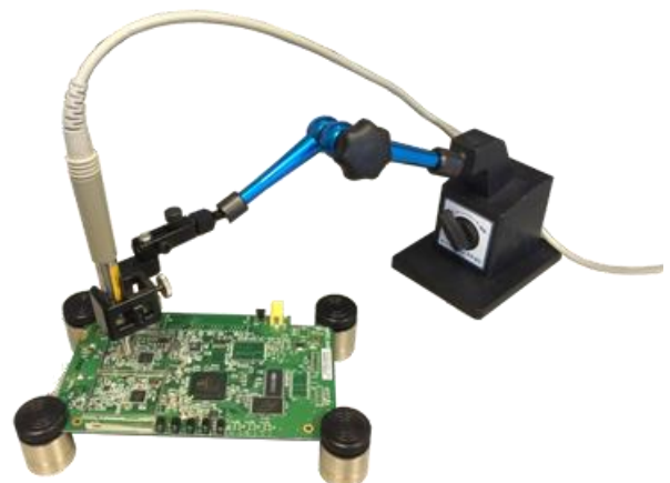
FP40-UA16 holding an RF Probe
