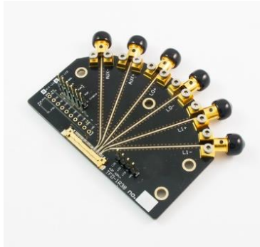
Figure 3-1. eDP 1.2 Receptacle 30pin Test Fixture
