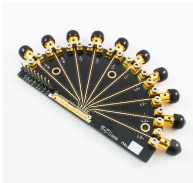
Figure 3-3. eDP 1.2 Receptacle 40pin Test Fixture
