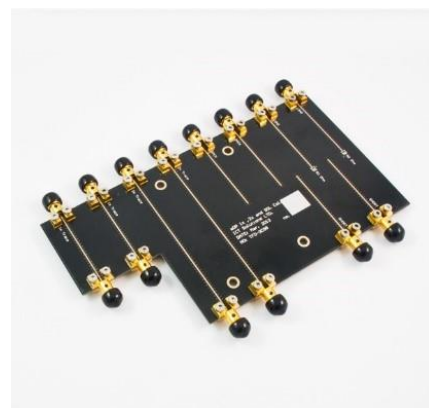
Figure 3-6. DP 1.2 1X,2X and SOL Calibration Board
