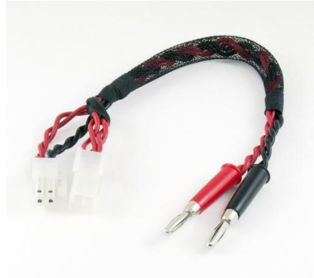
Figure 4-9. USB Type-C PD Cable Test Fixture
