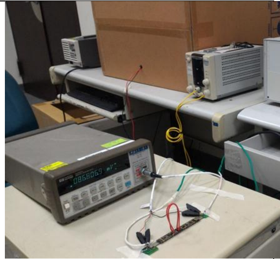
Figure 5-6. Low Level Contact Resistance and Voltage Drop
