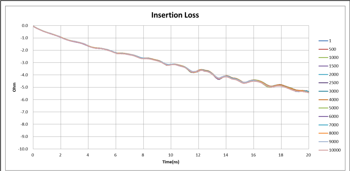
Figure 7-2. USB USB4 Type-C Receptacle High Speed Test Fixture Insertion Loss of SS-TX Pair
