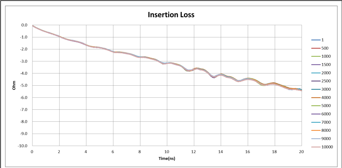
Figure 7-2. USB4 Type-C Receptacle High Speed Test Fixture Insertion Loss of SS-TX Pair
